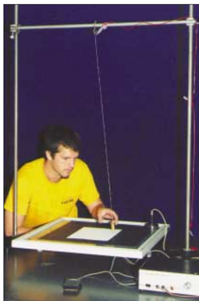
Fig. 1a. Photograph of UPS student Mike Dahl using the apparatus. The spherical pendulum is suspended above the air table and connected by magnet wire to the spark generator (right foreground.) The puck seen in the corner of the table is not mandatory, though it does provide a convenient way to complete the circuit from the carbon paper to the spark generator.
