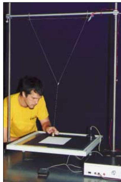
Fig. 1b. Photograph of the Y-suspended pendulum.
