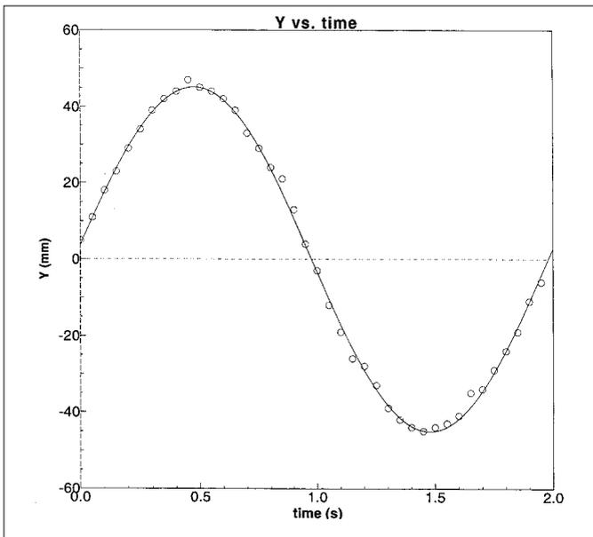
Fig. 2c.  $y(t)$  data (dots) plotted along with a sinusoidal curve fit (solid line). Measured pendulum length is  $L = 1.015$  m, giving theoretical period  $T = 2\pi(L/g)^{1/2} = 2.02$  s. Curve fitting of data yields  $T_x = 1.98$  s,  $T_y = 2.01$  s,  $\phi = 88^\circ$ .
