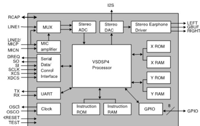
Figure 3: Block Diagram of VS1053 Decoder Chip
