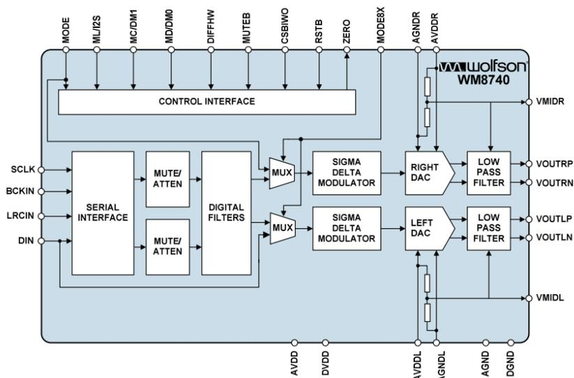
Figure 2: Block Diagram of WM8740 Stereo DAC
