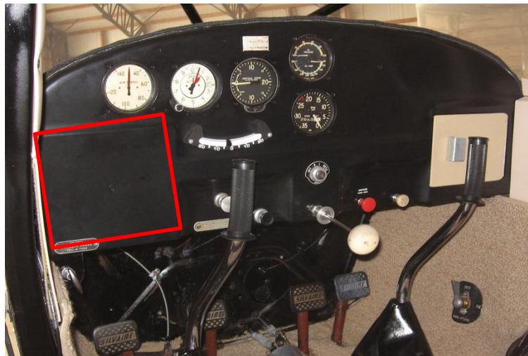
Figure 7: Luscombe Panel, installation location #1
