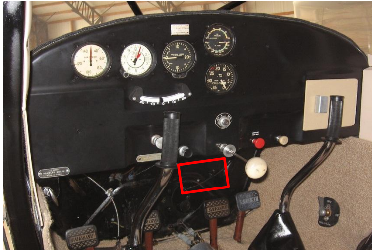
Figure 8: Luscombe Panel, installation location #2
