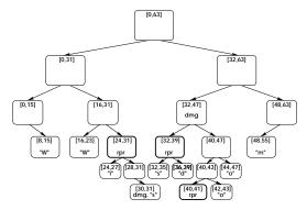
Fig. 5. Modified segment tree
