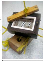
Figure 5. Field Device to hold glass slide tunicates in a Bay water setting at Fort Baker, CA.
