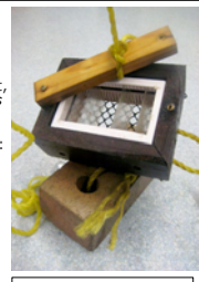
Figure 5. Field Device to hold glass slide settled tunicates in a Bay water setting at Fort Baker, CA.
