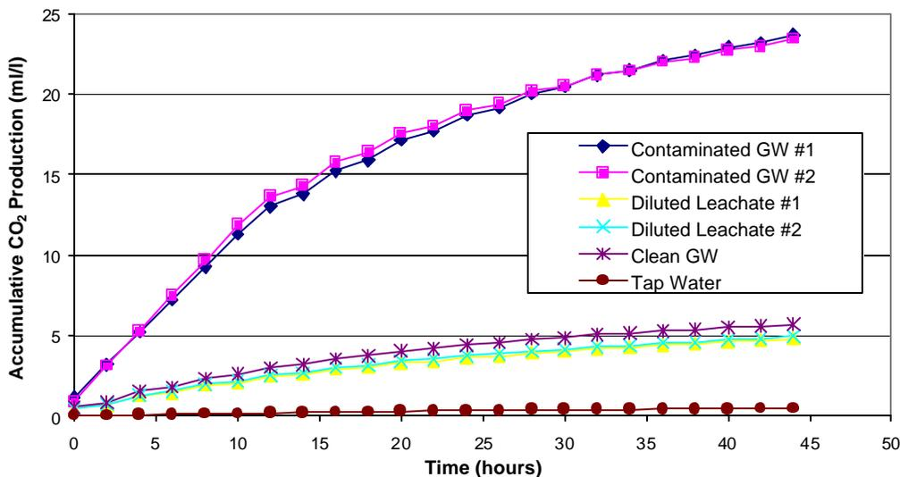
**FIGURE 3. Leachate accumulative CO<sub>2</sub> production from LTU2 compared to clean and contaminated groundwater – Week 1.**
