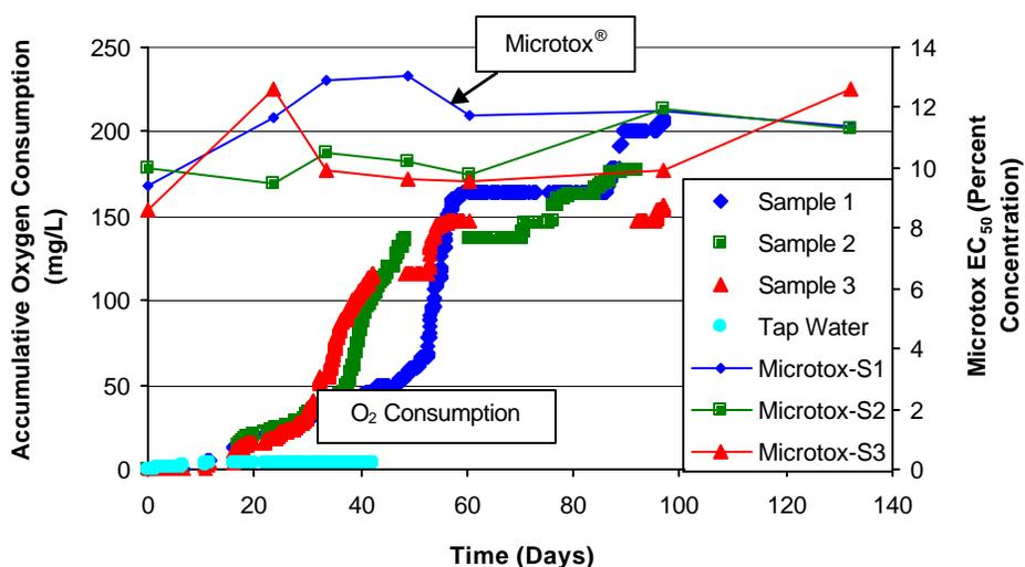
**FIGURE 1. Cumulative oxygen consumption and Microtox<sup>®</sup> toxicity for triplicate samples of leachate from LTU3 during Experiment 1.**
