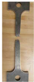
Figure 5. shows a steel 410 sample after applied tensile stress. Notice the necking caused in the middle where it broke.
