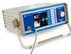
Figure 6. The Rollscan 300, which produces digital signal at multiple frequencies, measures Barkhausen Noise and collects data from each sample using the Microscan 600 software
