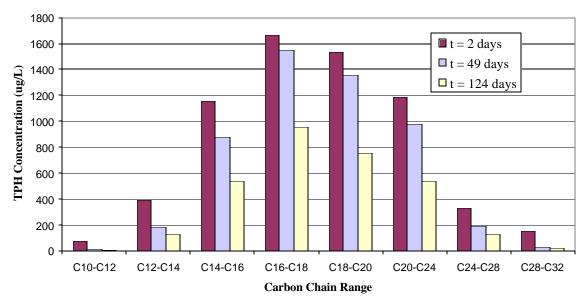
FIGURE 3. Simulated distillation of TPH concentrations in samples of experimental Bottle 1 groundwater at 2, 49, and 124 days.
