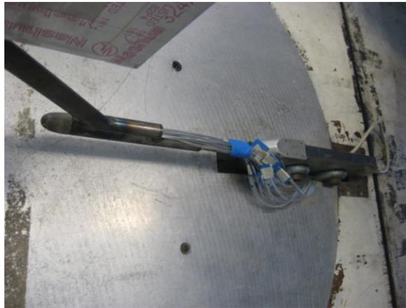
**Figure 7:** Pressure tubes routed into sting balance mount to the scannivalve.
