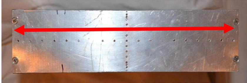
**Figure 3:** Spanwise pressure ports on backplate with no tabs.
