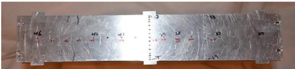
**Figure 5:** Spanwise pressure ports on backplate with tabs.
