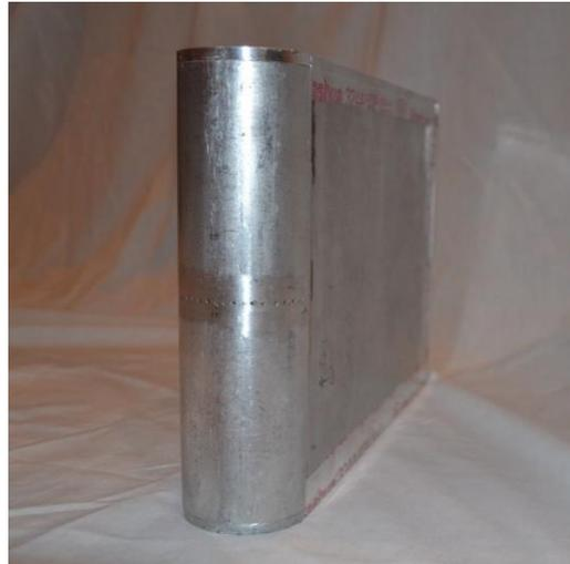
**Figure 1:** The 3D Bluff Body with a Blunt Edge Model Used
