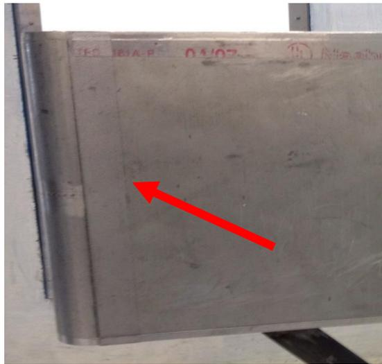
**Figure 4:** Rough strips used at leading edge.
