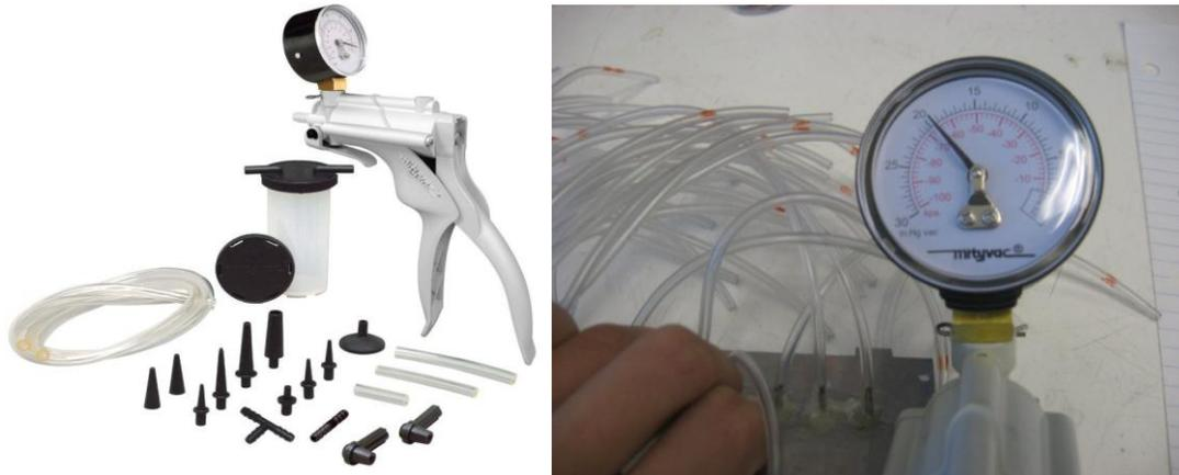
**Figure 8:** Handheld pressure pump (left) and pressure holding test for ports (right).
