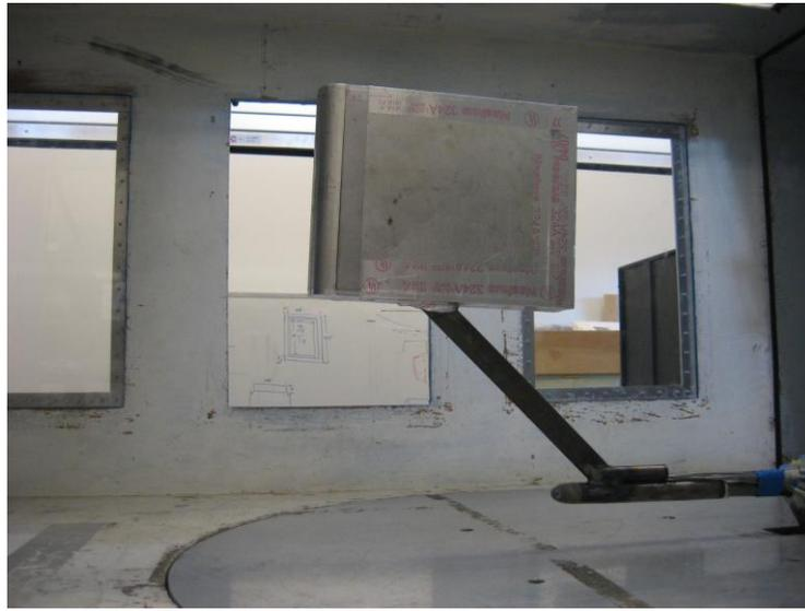
**Figure 12:** Model is shimmed at strut mount interface and streamlined with aluminum tape.
