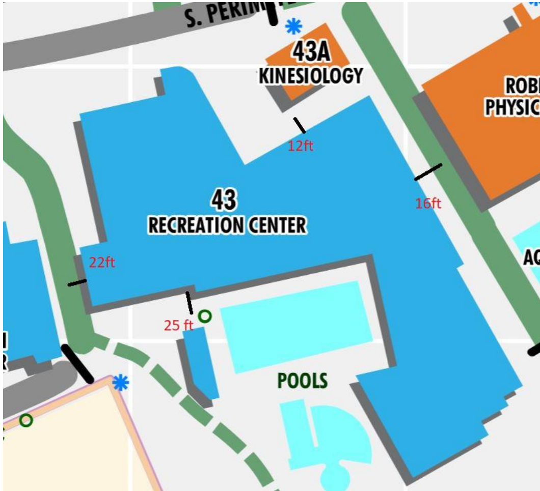
Figure 12. Fire Separation Distance
