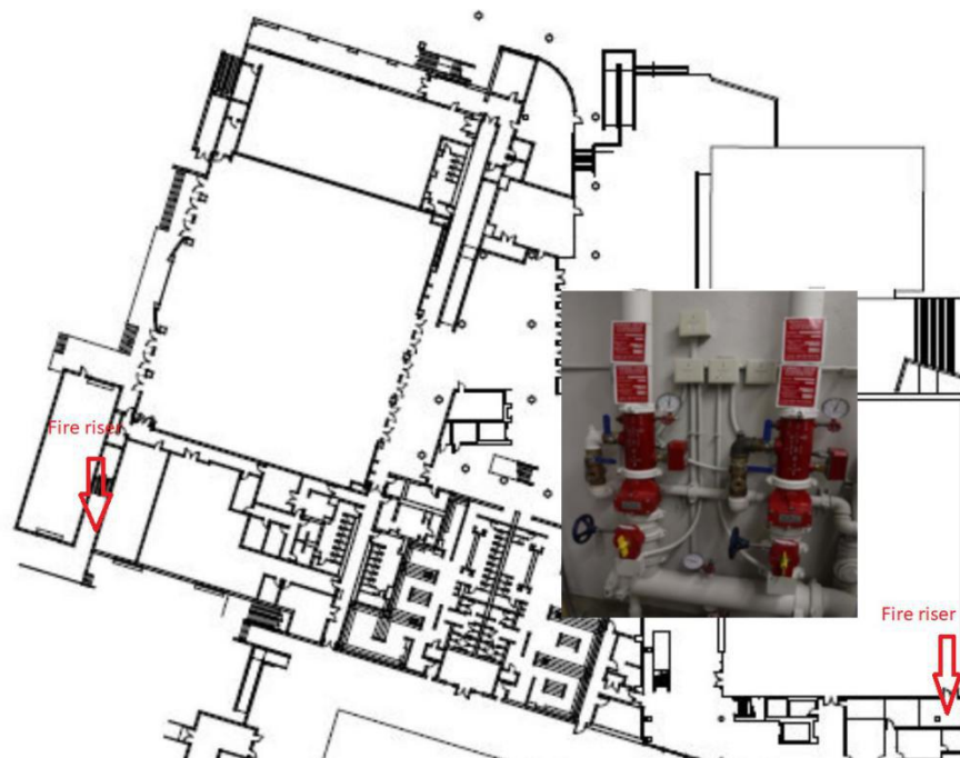
Figure 31. The Location of the Risers
