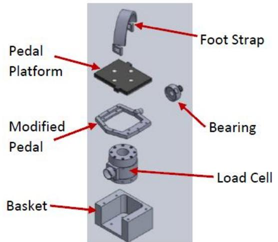
FIGURE 1. EXPLODED VIEW OF INSTRUMENTED PEDAL DESIGN.
