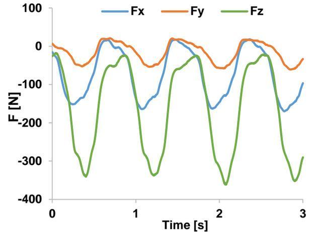
**FIGURE 1. MEASURED FORCES ACTING ON THE PEDAL FROM ONE SUBJECT. USING THE COORDINATE SYSTEM SHOWN IN FIG. 2B, THE -X, -Y, AND -Z VALUES CORRESPOND TO FORCE (F) COMPONENTS IN THE POSTERIOR, LATERAL, AND DISTAL DIRECTIONS.**
