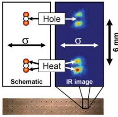
CFRP bar with drilled holes
