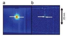
Fig. 5. (a) Raw infrared (IR) heating data compared to (b) processed IR data isolating regions of heat generation along the crack and at the crack tips.
