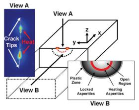
Fig. 2. Hypothesized schematic of how heat is generated in a semielliptical surface crack. View A shows the measured surface heating of the crack and View B shows the cross-section of the crack as observed when the crack is broken open. The superimposed dotted line in View A shows crack length and the white arrows point to the crack tips.
