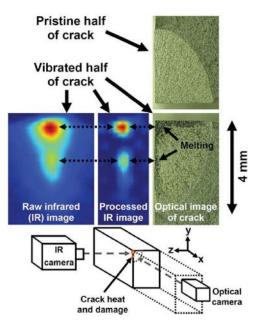
Fig. 4. Correlation of frictional heat generation with crack face damage in titanium (Ti 6-4), (top, right) an optical image of the unvibrated half of the crack; (middle, left) raw heating data after 1.0 s of excitation; (middle, center) processed heating data isolating regions of heat generation, (middle, right) melting and other damage observed on the crack faces; and (bottom) a schematic of the crack and sample geometry.
