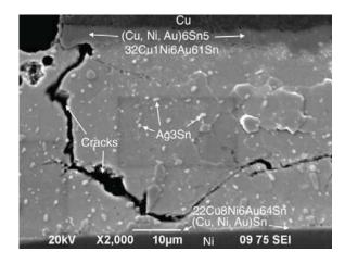
Fig. 4. Fracture in bulk solder of a QFN on a flash Au board, after thermal aging for 56 days.
