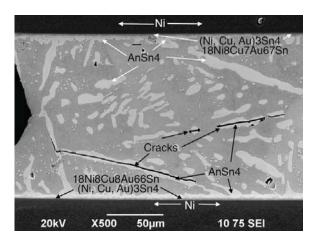
Fig. 7. Fracture in AuSn<sub>4</sub> IMC in the bulk solder, a TOPS component on a thick Au board, after thermal aging for 30 days.
