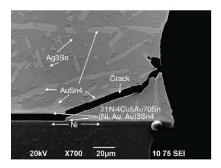
Fig. 8. Fracture in the IMC near the board side, a TOPS component on a thick Au board, after thermal aging for 30 days.
