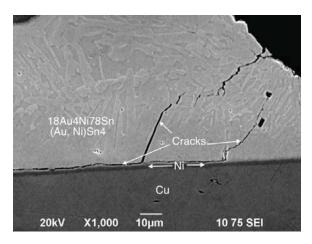
Fig. 12. SEM images of solder joints of an FP component on a flash Au board, after thermal aging for 56 days.
