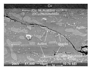
Fig. 6. Fracture in AuSn<sub>4</sub> IMC in the bulk solder, a QFN component on a thick Au board, after thermal aging for 56 days.
