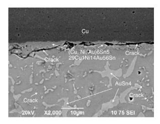
Fig. 5. Fracture in bulk solder joint and IMC near component side, a QFN on a thick Au board, as-built.
