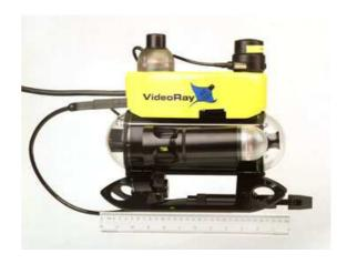
Figure 11: The VideoRay Pro III Micro ROV.
