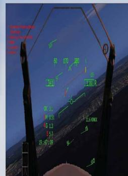
Distorted by display configuration, apparently 45° bank angle\*
