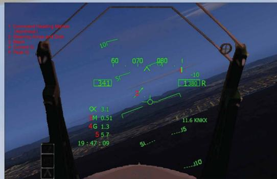
Undistorted simulated image (25° tilted horizon)\*
