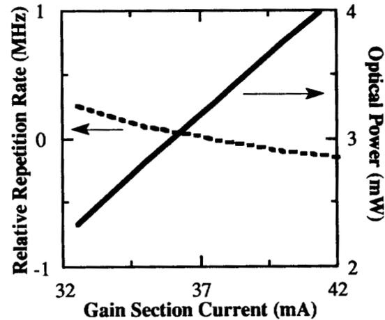
Figure 2. Measured repetition frequency tuning using control of gain section current and absorber section voltage.
