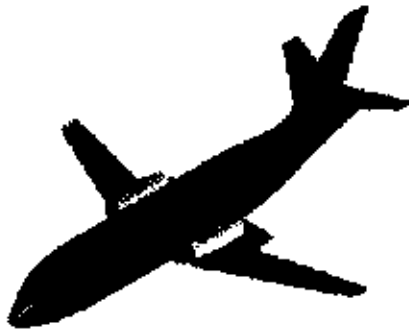
Figure 1. Configuration 1 is comprised of a high aspect ratio wing, over the wing engines, circulation control at the trailing edge and a cruciform tail.
