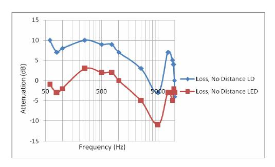
Figure 5: Attenuation of each source compared to direct speaker connection
