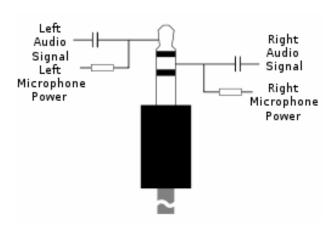
Figure 3: TRS Connector Diagram
