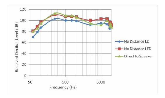
Figure 4: Comparison of transmission using light sources to direct speaker connection
