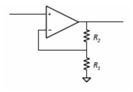
Figure 1: Non-inverting Amplifier Configuration
