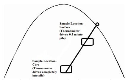
**Figure 3.** Cross section of compost pile-location of temperature and sample collection.
