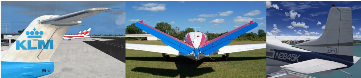
Figure 5. T-tail, V-tail, and Conventional tail
