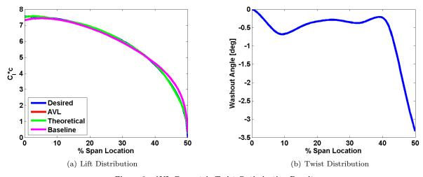
Figure 8. AVL Geometric Twist Optimization Results
