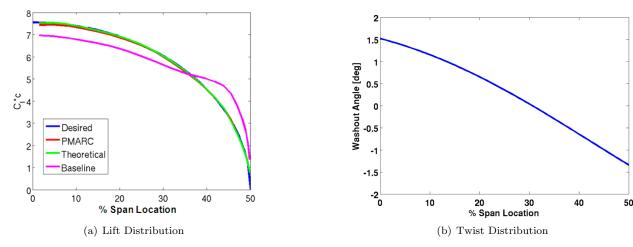
Figure 9. PMARC Geometric Twist Optimization Results
