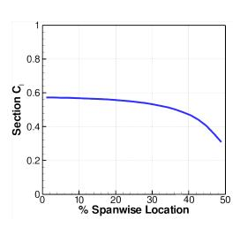
Figure 5. Lift Distribution of Untwisted Wing
