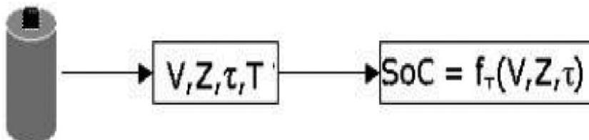
Where SoC is state of charge, and the variables such as battery voltage (V), battery impedance (Z), and the voltage relaxation time ( $\tau$ )
