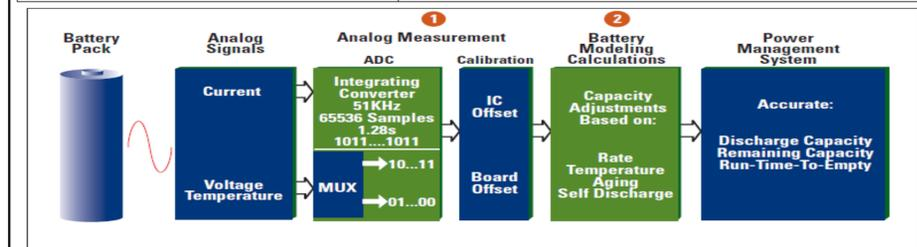
The two components of battery fuel gauge accuracy depend on analog measurement and battery modeling.
