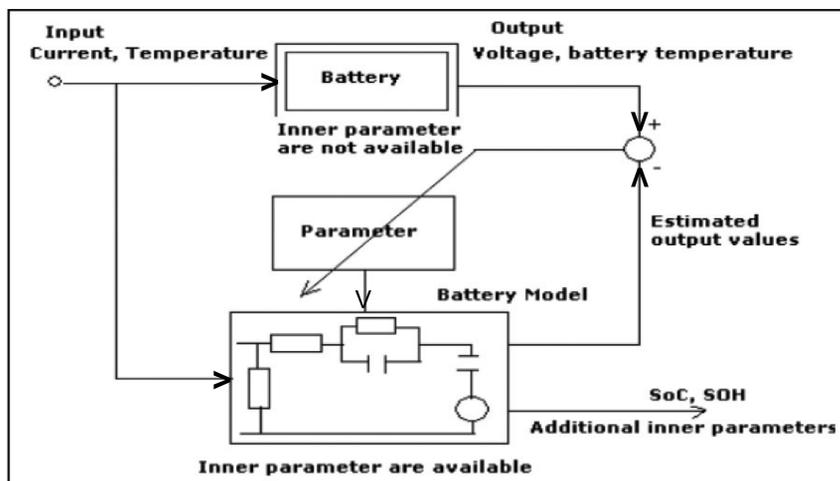
RSOC determination using Kalman filter.
