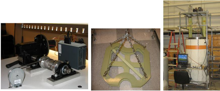
**FIGURE 2.** (Left) This image shows the mechanical setup of the lowering mechanism including the stepper motor connected to a 50:1 worm gear reducer and the stepper motor controller electronics. (Middle) Lowering platform made of G-10 capable of holding a 76.2 cm racetrack coil. (Right) The thermal cycle test apparatus.
