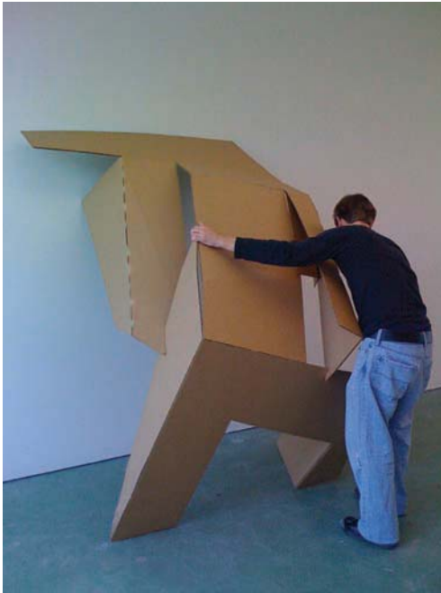
Testing at Full Scale: While a compelling solution at model scale, at full scale the solution was too light and flexible. ▼
