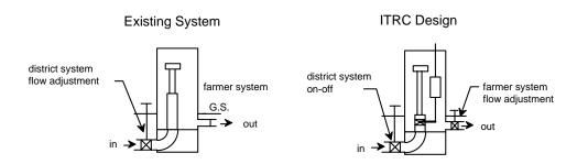
Figure 2. Existing Turnout and First Pressure Regulator Design.
