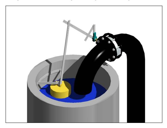
Figure 3. Present Design of an Up-and-Over Pressure Regulator for DEID.
