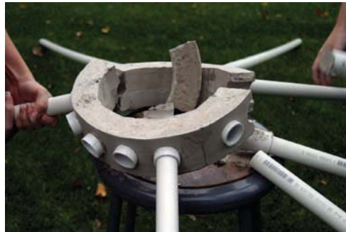
Critical Joint: failed joint study in concrete, ▲ ▼ successful joint in wood. Barn Raising: bending PVC structure involved ▶ cooperation from multiple teams to raise in one lift.
