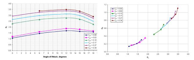
Figure 22. Lift Due to Angle-of-attack for Dual Radius Flap Deflection Angle = 60°
