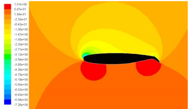
Figure 13. Pressure Coefficient Contours for C_{\mu} = 0.05 , Angle-of-Attack = 6^{\circ} and Flap Deflection = 30^{\circ}
