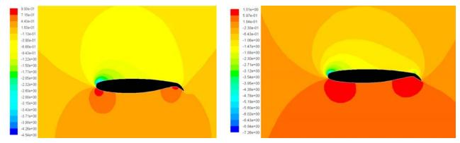
Figure 12. Pressure Coefficient Contours for  $C_{\mu}$  = 0.00, Angle-of-Attack = 6° and Flap Deflection = 30°
