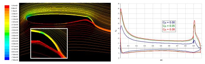
Figure 16. Path Lines Colored by  $C_P$  for  $C_{\mu} = 0.08$ , Angle- Figure 17. Pressure Coefficients for Angle-ofof-Attack =  $6^{\circ}$  and Flap Deflection =  $30^{\circ}$
