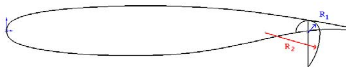
Figure 4. Baseline NASA SC(2)-0414 Supercritical Airfoil with Superimposed Dual Radius Flap, R_1/c = 0.0341 , R_2/c = 0.1544
