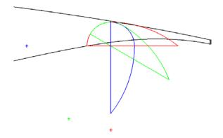
Figure 5. Dual radius Flap Positions, Red =  $0^{\circ}$ , Green =  $30^{\circ}$ , Blue =  $90^{\circ}$  and original SC(2)-0414 (Black)
