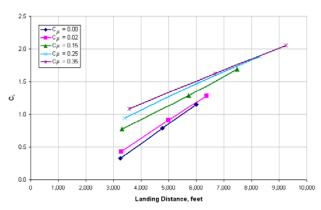
Figure 30. Landing Distance for Dual Radius Flap Deflection Angle =  $0^{\circ}$
