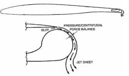
Figure 1. Basic Circulation Control Configuration with Trailing Edge Detail<sup>1</sup>
