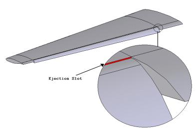
Figure 8. Solid Model of Circulation Control Wing with Ejection Slot Detail
