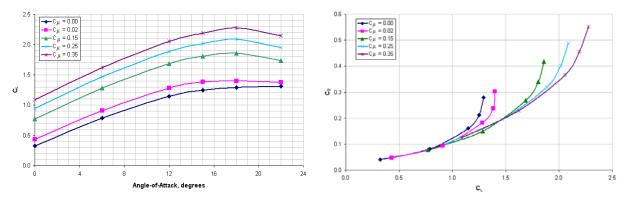
Figure 18. Lift Due to Angle-of-Attack for Dual Figure 19. Radius Flap Deflection Angle =  $0^{\circ}$
