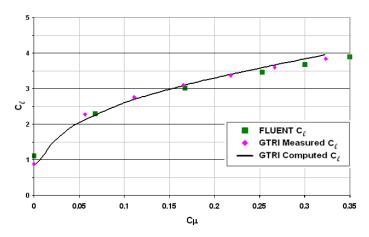
Figure 11. Two-Dimensional Lift Comparison with GTRI Data
