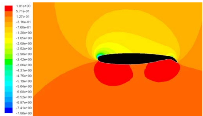
Figure 15. Pressure Coefficient Contours for C_{\mu} = 0.08 , Angle-of-Attack = 6^{\circ} and Flap Deflection = 30^{\circ}
