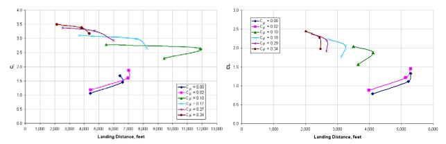
Figure 32. Landing Distance for Dual Radius Flap Figure 33. Landing Distance for Dual Radius Flap Deflection Angle =  $60^{\circ}$
