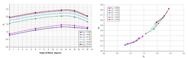
Figure 24. Lift Due to Angle-of-attack for Dual Radius Flap Deflection Angle = 90°
