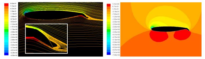
Figure 14. Path Lines Colored by  $C_P$  for  $C_{\mu} = 0.00$ , Angle-of-Attack = 6° and Flap Deflection = 30°
