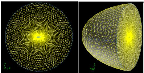
Figure 10. a) Meshed Plane-of-Symmetry (left) and b) Meshed Volume (right)
