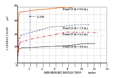
Fig. 1 - Test Panel Load Deflection Characteristic
