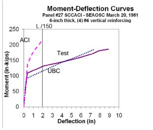
Fig. 2 – ACI and UBC Comparison to Test Data
