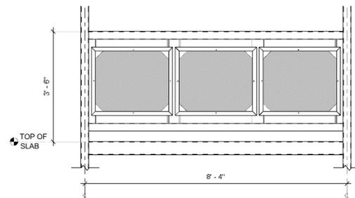
Figure 1: Exterior Guardrail (Typical)
