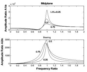
Figure 9 Response curves for various locations of disk. Ro=0.5, ao=180°
