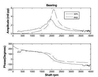
Figure 5 Synchronous response of a bowed rotor at outboard bearing. Ro=.64, ao= 180 °.
