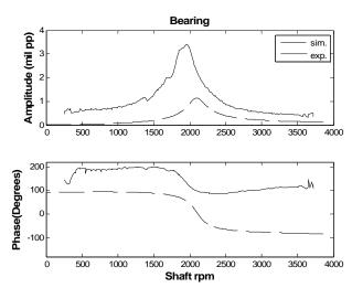
Figure 7 Synchronous response of a bowed rotor at outboard bearing. Ro=1.09, ao = 180 degrees.
