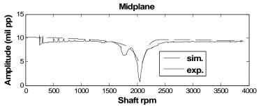
Figure 3 Bowed rotor experimental (exp.) and simulated (sim.) response.
