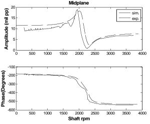
Figure 6 Synchronous response of a bowed rotor at midplane disk. Ro=1.09, ao = 180 °.
