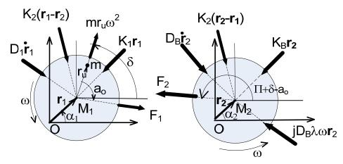
Figure 2 Lumped parameter modeling of forces in each plane.
