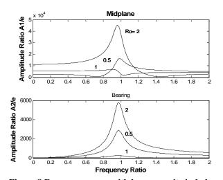
Figure 8 Response curves with bow opposite imbalance for various bow factors, Ro
