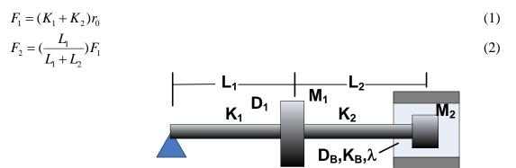
Figure 1 Two mass flexible rotor model
