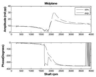
Figure 4 Synchronous response of a bowed rotor at midplane disk. Ro=.64, ao = 180°. Drop out of data near 2000 rpm is due to displacement exceeding transducer range. Phase wrap evident in the experimental plot around 1700 rpm and above 3500 rpm is due to software that adds 360° for phase ranges beyond 360°
