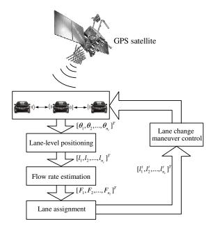
Fig. 4. Control diagram:  $[\theta_1, \theta_2, ..., \theta_{n_c}]^T$  are the GPS measurements for car 1 through car  $n_c$ ,  $[l_1, l_2, ..., l_{n_c}]^T$  are their lane positions,  $[F_1, F_2, ..., F_{n_l}]^T$  are the estimated flows in lane 1 through lane  $n_l$ , and  $[l_1^t, l_2^t, ..., l_{n_c}^t]^T$  are target lanes for these cars.
