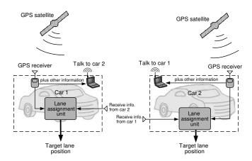
Fig. 2. Architecture for inter-vehicle communication.
