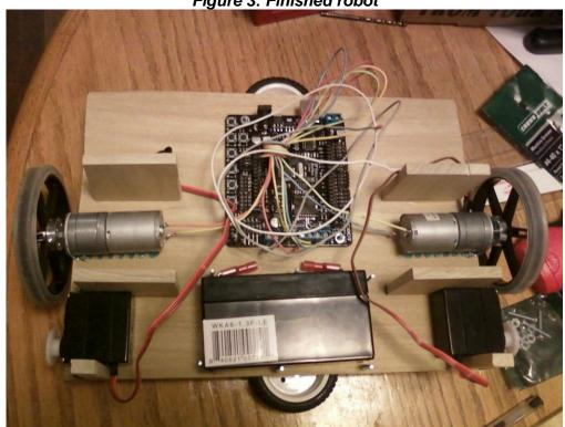
Figure 4: Servos and motors attached to Romeo controller
