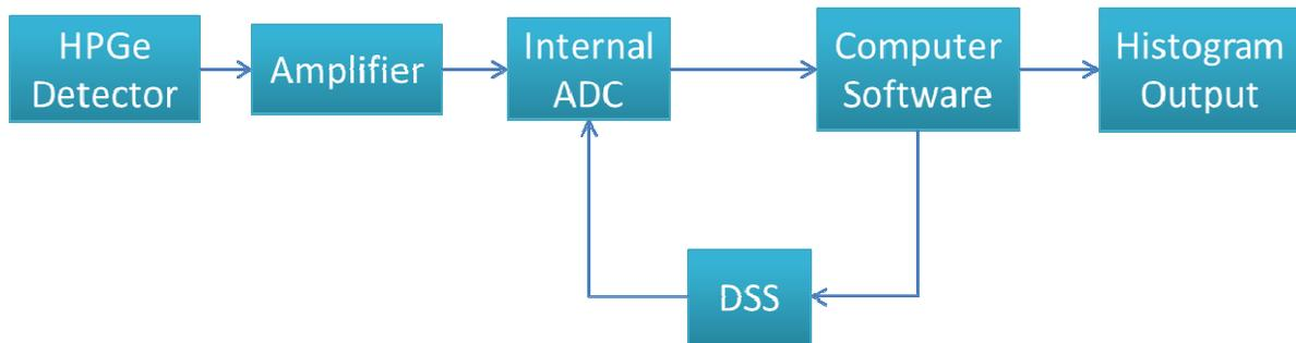
Figure 4. Functional block diagram of HPGe gamma ray spectrometer.
