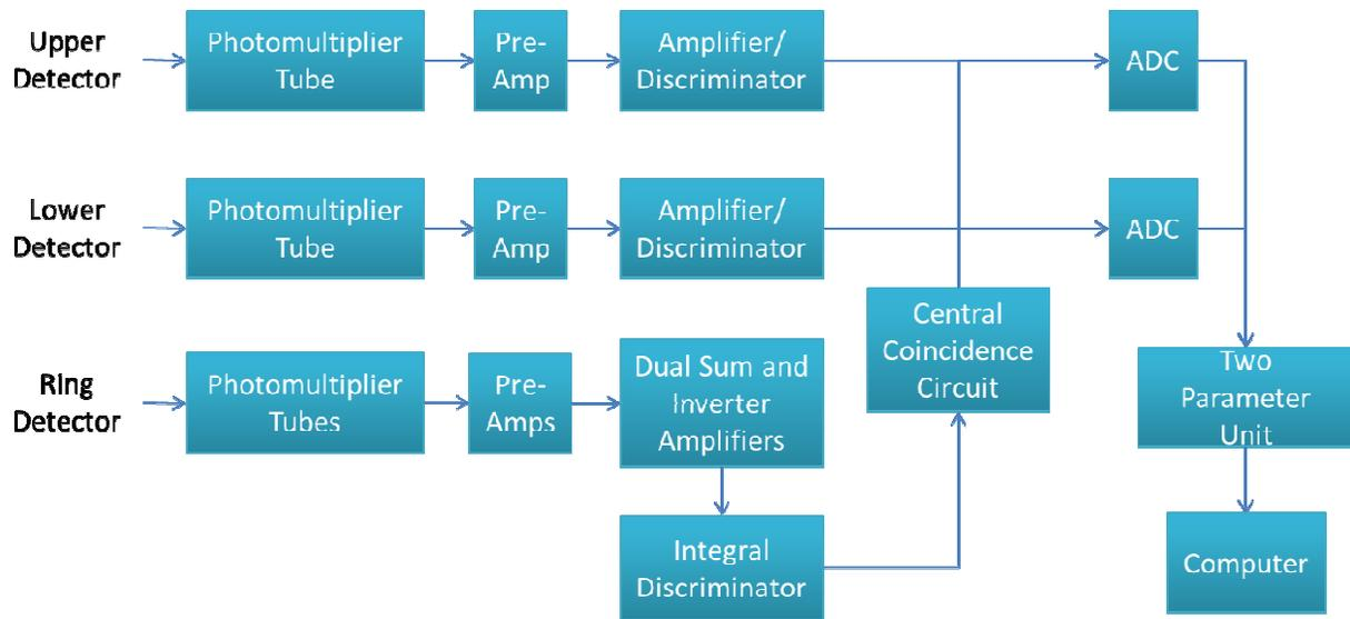
Figure 2. Functional block diagram of the MGRS.
