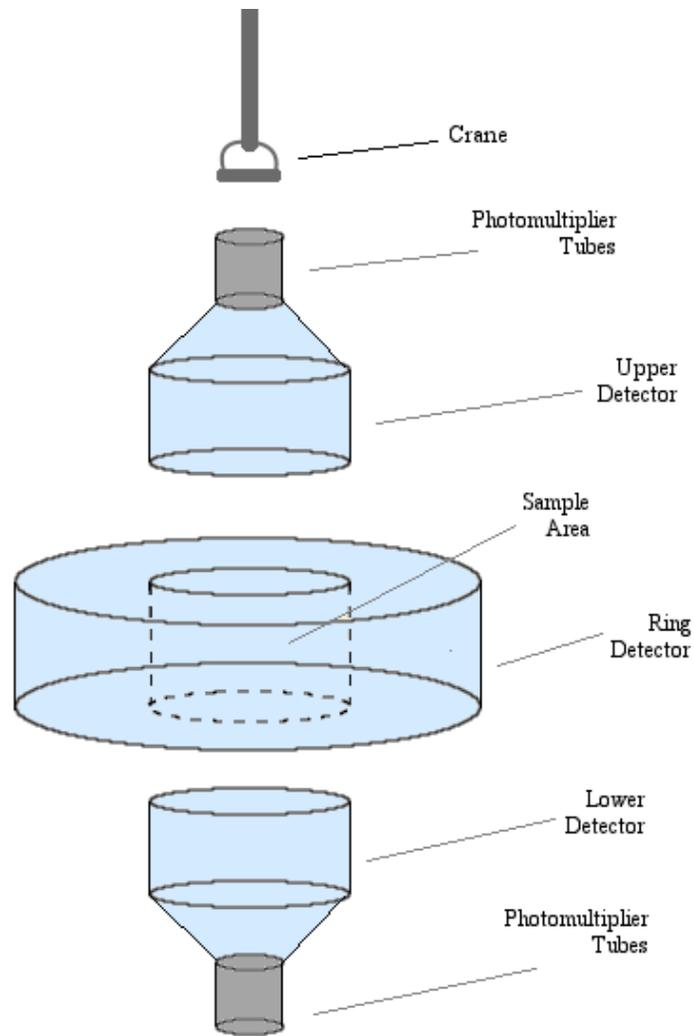
Figure 1. Schematic of multidimensional gamma ray spectrometer. Ring photomultiplier tubes are not shown along with other hardware and housing.
