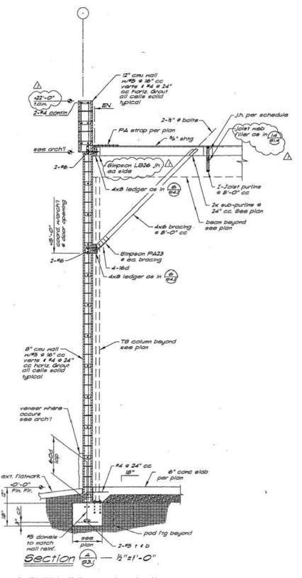
Figure 8: CMU building section detail
