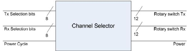
Figure 6 - Channel Selector Hardware diagram
