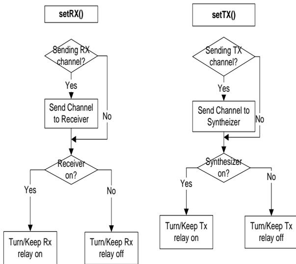
Figure 19 - setRX and setTX Software Flowcharts
