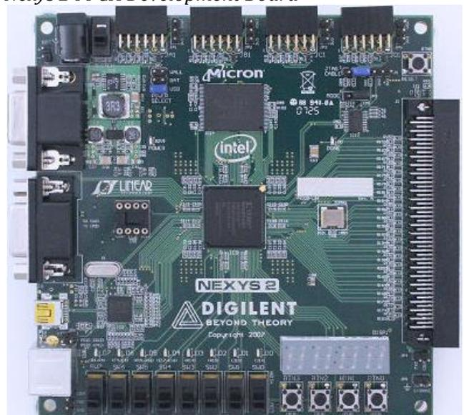
Figure 24 - Nexys 2 FPGA Development Board
