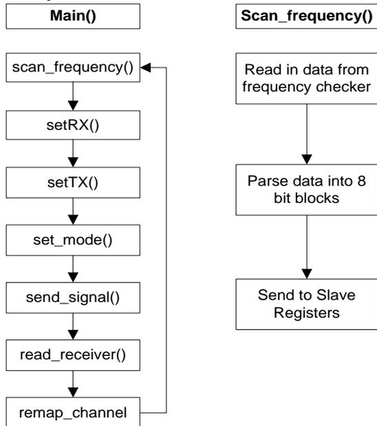
Figure 18 - Scurvy Main and Scan\_Frequency software flowcharts
