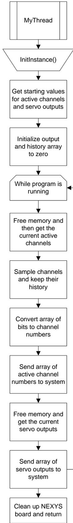
Figure 13 - MyThread Software Flowchart
