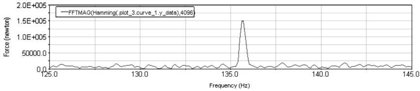
From the contact forces, we can get the meshing frequencies by FFT.
