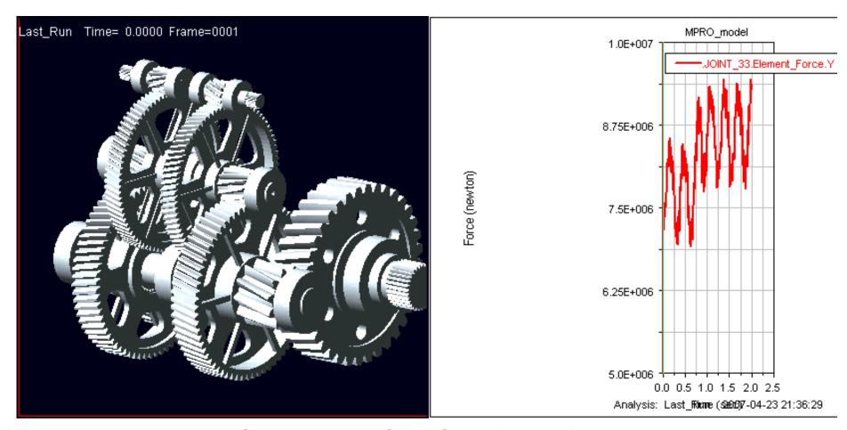
The crawler travelling system is driven by a three-stage gear transmission.
