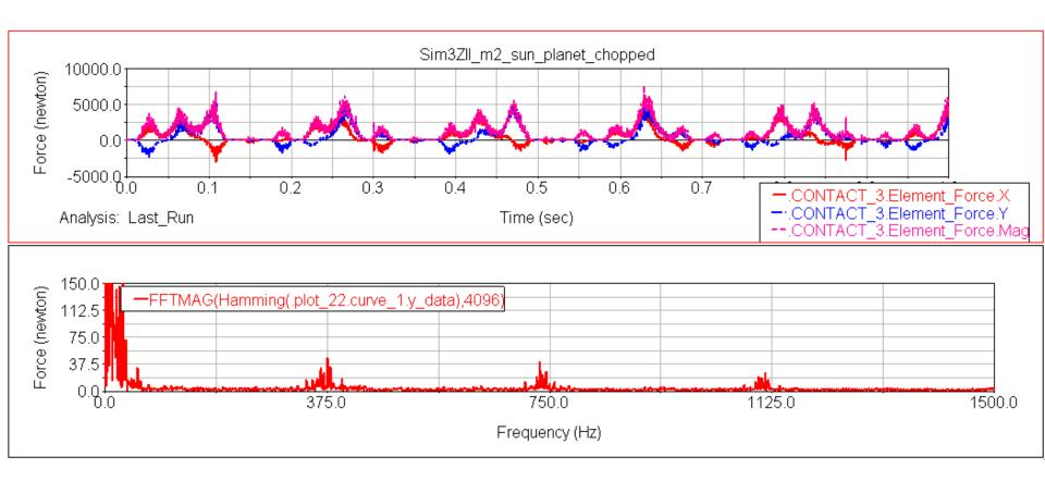
The hunting tooth frequency shows up when teeth malfunction occurs on both pinion and gear.
