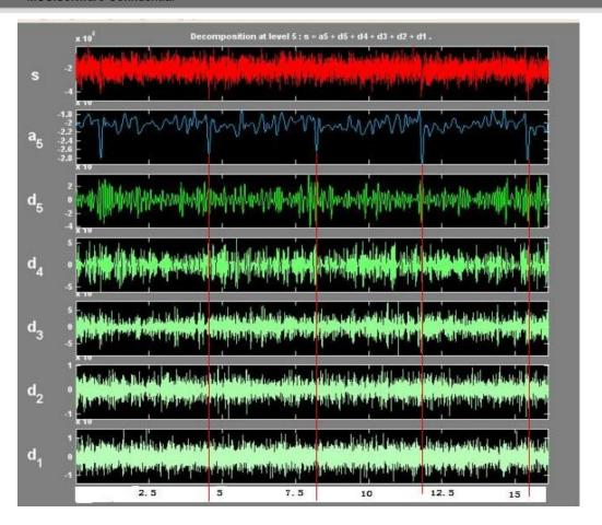
To simulate the fault mode of gearbox, a pinion with chopped tooth joints in the ADAMS model, and the meshing frequency of the fault tooth of the pinion can be detected by wavelet transform after the contact force simulation.
