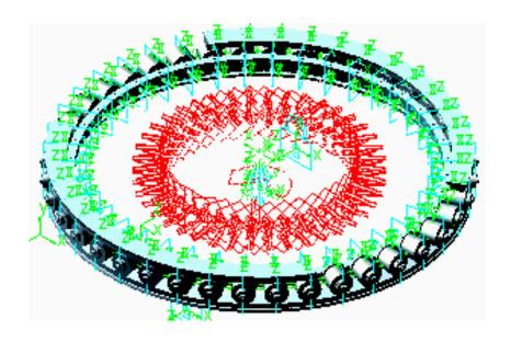
To perform simulation, the driving torque and braking torque are applied to the upper structure along with the upper tracks, and the contact forces are applied between rollers and tracks.
