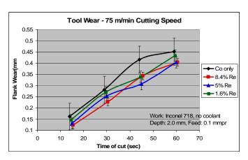
FIGURE 3 INCONEL 718 WEAR TESTS AT 75 M/MIN
