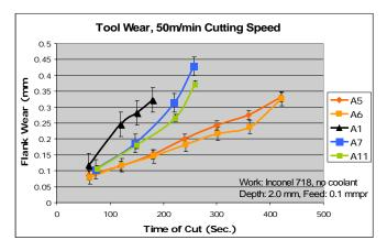
FIGURE 6 TOOLS A1, A5, A6, A7, A11 RUN TO FAILURE
