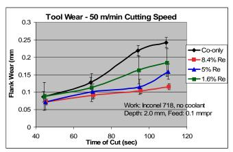
FIGURE 2 INCONEL 718 WEAR TESTS AT 50 M/MIN
