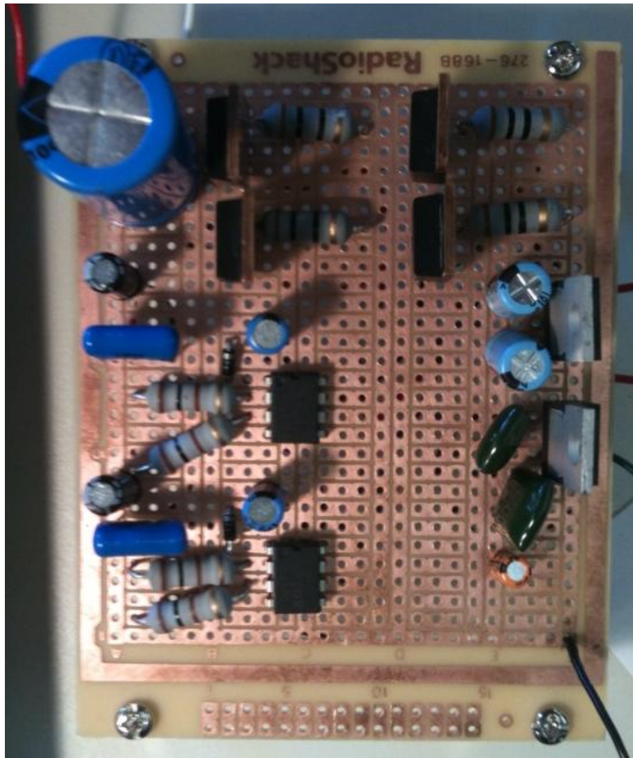
Figure 5-2: Prototype Board with Soldered on Components
