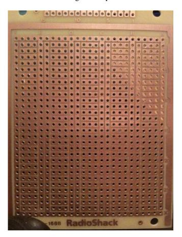
Figure 5-1: Blank Prototype Board with Copper Traces
