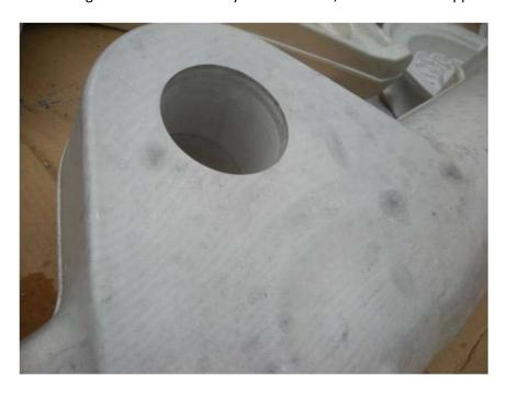
Figure 1 - Finished Weber forging showing bands of high- and low-solute regions, an artifact from macrosegregation at the surface of the ingot.
