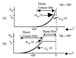
Figure 2 Normal and Shear Stresses on Wear Land for a)  $VB < VB^*$ , b)  $VB > VB^*$
