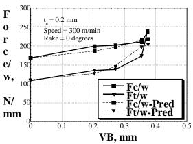
Figure 3 Predicted and Measured Wear Forces - KC730 Tools (VB\* = 0.25 mm)
