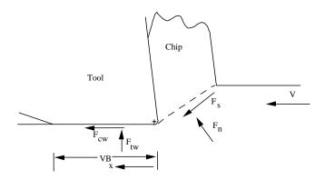
Figure 1 Cutting Tool with Flank Wear Land
