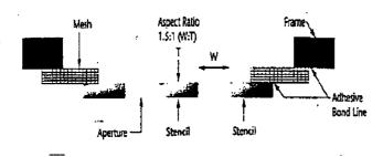
Figure 1. The aperture aspect ratio, or the opening's width to stencil thickness. The minimum (1.5 W to 1.0 T) will influence the latter.
