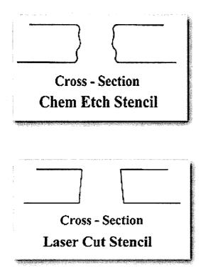
Despite the advances brought on by the use of lasers in stencil technology, the approach can be costly. For large production quantities, the
