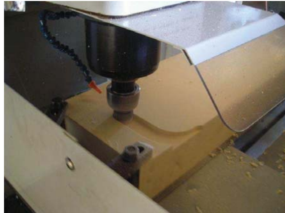
Figure 2: CNC mill used for the manufacturing of rapid prototype composite blade. (Courtesy of Mr. B. Edwards, MS student)
