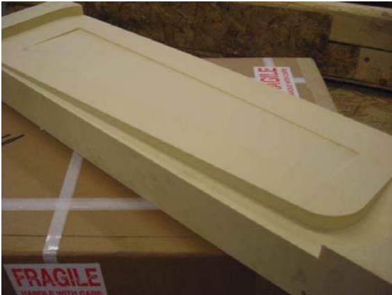
Figure 3: Completed female mold (Courtesy of Mr. B. Edwards, MS student)
