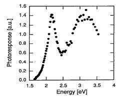
FIG. 4. Spectral response of the photocurrent in ITO/MEH-PPV/ $C_{66}$ /Au photodiode at (reverse) -1 V bias.
