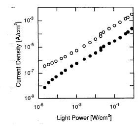
FIG. 3. Short circuit current (closed circles) and photocurrent at -1 V bias (open circles) as a function of light intensity for the ITO/MEH-PPV/C<sub>60</sub>/Au device.
