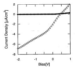
FIG. 2. Current vs voltage characteristics of the ITO/MEH-PPV/ $C_{60}$ /Au device in the dark (diamonds) and upon illumination with the 514.5 nm line from an argon ion laser of  $\approx 1$  mW/cm<sup>2</sup> (triangles).
