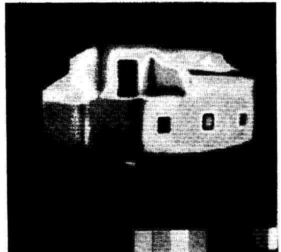
*Left:* A model of a house constructed by students Jeff Kepple and Ted Trouard. The effects of various glazings, insulations, and materials (black chrome, etc.) are easily accessible to infrared measurements by the architecture students. *Right:* Note that the infrared image of the house has been reversed.
