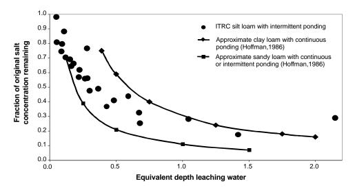
Figure 6. Relationship between the equivalent depth of leaching water and the fraction of initial salt content, considering five inner soil cores (modified).
