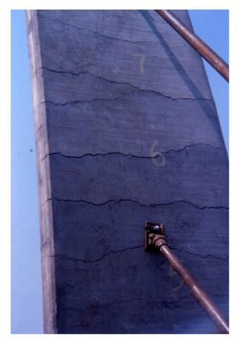
Fig. 5 – Test Panel Showing Cracking Pattern
