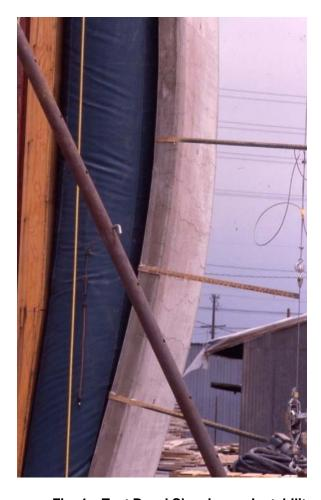
Fig. 4 – Test Panel Showing no Instability
