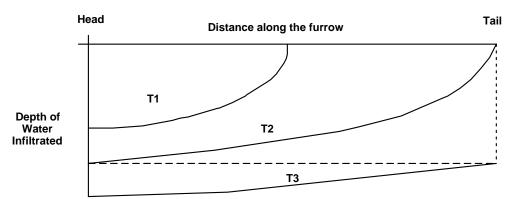
Figure 3. Depths of water infiltrated at various distances along a furrow at three times (T1, T2, and T3). T3 = 2 T2. The dashed horizontal line indicates the depth of water needed if perfect irrigation scheduling occurred. Assumes a uniform soil.
