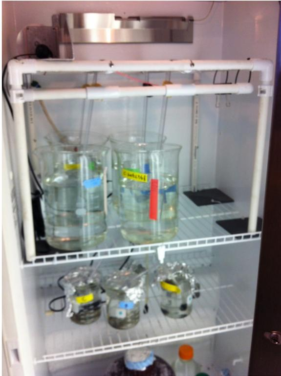
Figure 1. Cultures of larvae (above) and egg capsules (below) in an incubator. Larvae are stirred by a continuous swinging paddle apparatus, built by Megan Wilson and Biology department technicians.
