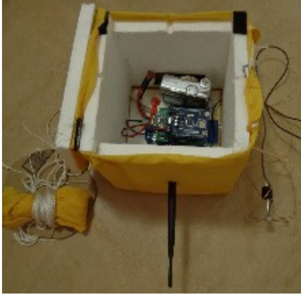
Figure 10. Payload box with interior components, antennas, and parachute.
