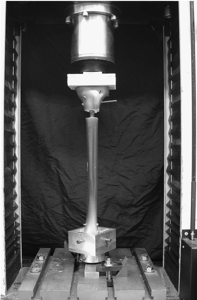
FIGURE 2. Experimental testing of a tibia-implant construct in axial loading.
